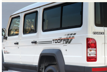
New longer, wider, pressed panel steel body with concealed door hinges.
