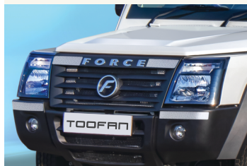
New front fascia, new headlamps, new bumpers with integrated fog lamps.
