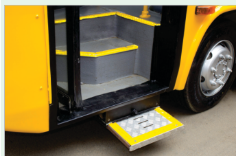
Low foot step and Hand Rail for easy entry & exit
